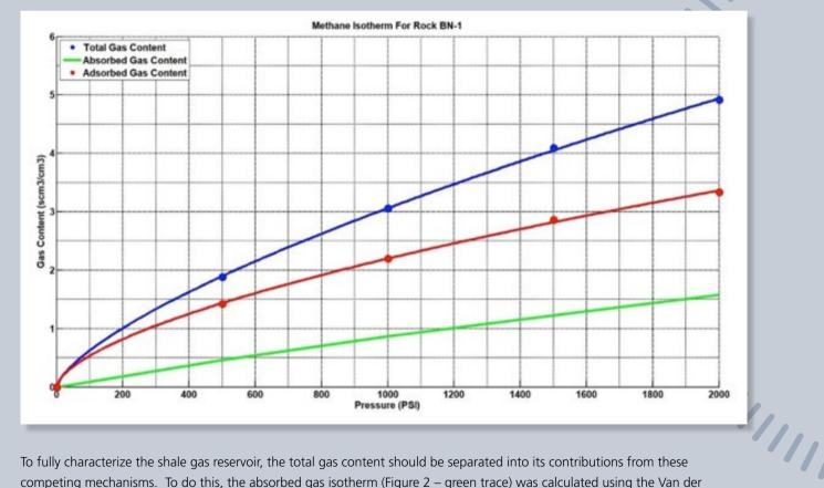
To fully characterize the shale gas reservoir, the total gas content should be separated into its contributions from these competing mechanisms. To do this, the absorbed gas isotherm (Figure 2 – green trace) was calculated using the Van der Waals equation and the pore volume of the rock. The adsorbed gas isotherm (Figure 2 – red trace) was then derived by subtracting the absorbed gas isotherm from the total gas isotherm.
