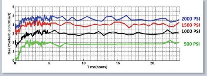
The total gas content of the shale for each pressure as a function of time is shown in Figure 1. This figure shows that it takes two to four hours for the methane to fully infiltrate the shale core plug. Following this initial stabilization, the gas content is constant over the remainder of the experiment. Other experiments, with other types of rocks, have shown that this stabilization period is rock dependent.
